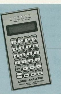
YOU CAN NOW ADD LOGIC ANALYZERS to the list of electronics test equipment that has made the transition from being esoteric and expensive to being rudimentary and relatively inexpensive. As microprocessor-based equipment became ubiquitous, having the proper tools to service them became essential to technicians. Helping to fill that need was a handheld, 16-channel, 20 MHz logic analyzer from Precision Motion (3563 Sueldo Building J, San Luis Obispo, Ca 93401).
